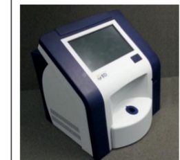
Figure 5: BD's POC HNW instrument for low resource settings. Instrument is controlled via an on-board CPU.
