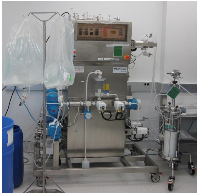
Chromatography Skid with Product and Buffers (bags) and Column
