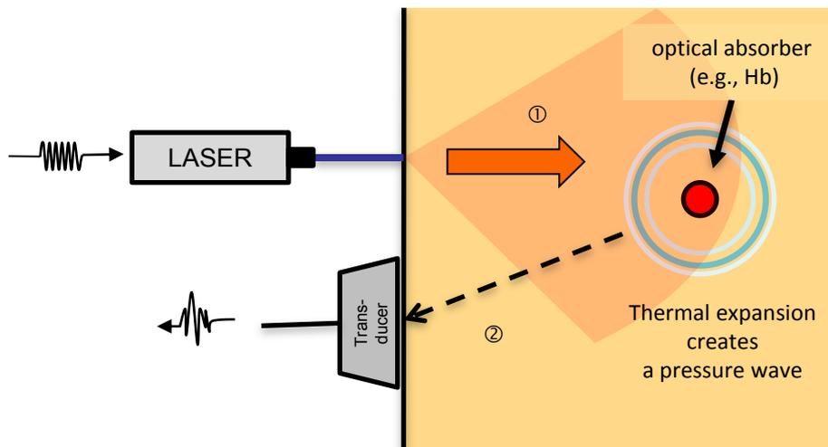
**Nexus 128:** uses a tunable laser and 128 acoustic receivers to produce multi-spectral images, in less than 1 minute
