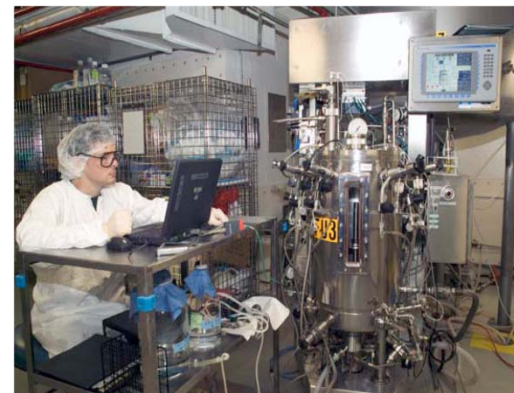
GMP 80L fermentation of rhIL-15: Production and pooling of several of products from several fermentations needed for one 1gram lot of rhIL-15
