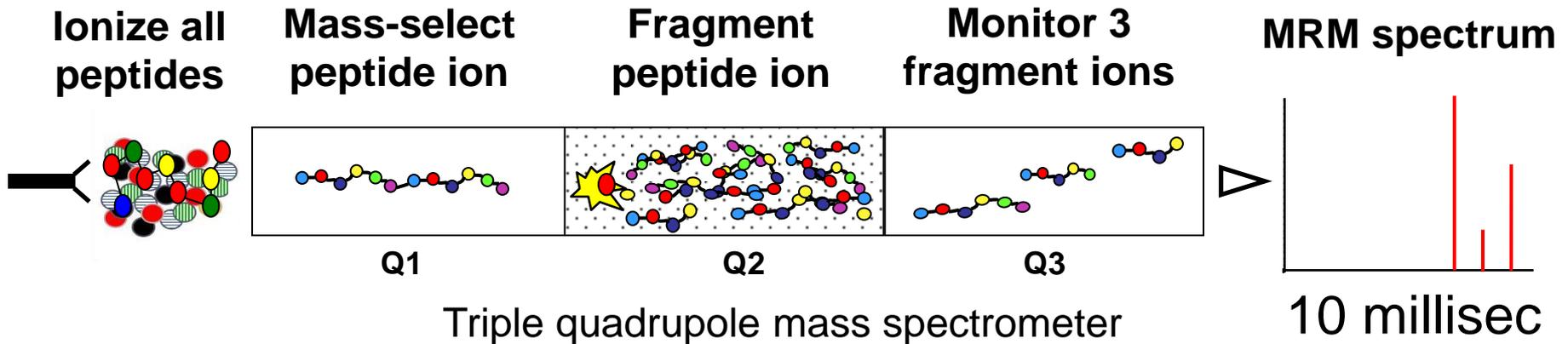
Triple quadrupole mass spectrometer
